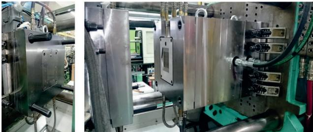
Figure 152: Improved core-back mold mounted on Arburg 470 machine
