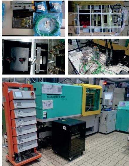
*Figure 159: Mold and components for external core-movement (upper), initial experiments (middle) and final experimental setup including all electrical devices and computer in an external box (lower)*
