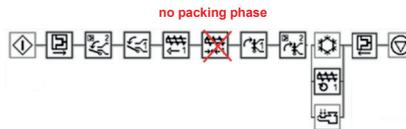
Figure 22: Process sequence for low-pressure foam injection molding procedure (LP-FIM); (start of cycle -> closing mold -> open nozzle mold -> open nozzle plasticizing unit -> injection -> no packing pressure -> close nozzle plasticizing unit -> close nozzle mold -> cooling – parallel: dosing material and injection of gas -> opening of mold and ejection -> end of cycle
